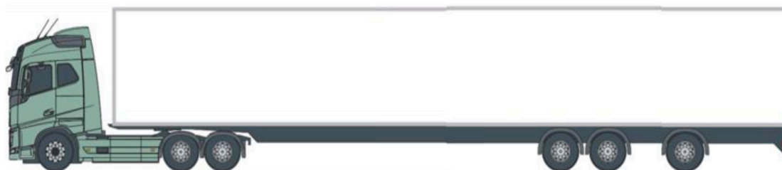
Figure 6. 6-axis articulated vehicle (max. 17.5 m), modified from 19 .
