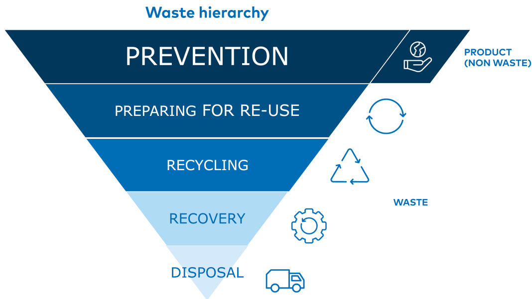
Figure 2: The Waste Hierarchy as described in the EU Waste Framework directive. [2]
